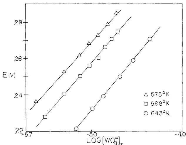
Figure 1.—Oxygen electrode potentials as a function of total tungstate concentration at several temperatures. Observed and calculated slopes for the different temperatures are, respectively:  $575^\circ\text{K}$ , 0.0576 v, 0.0569 v;  $596^\circ\text{K}$ , 0.0593 v, 0.0590 v;  $643^\circ\text{K}$ , 0.0625 v, 0.0638 v.
