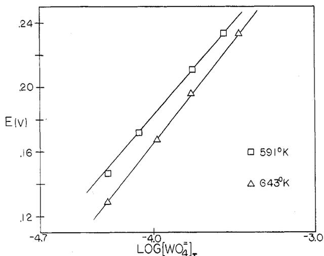
Figure 2.—Oxygen electrode potentials as a function of total tungstate concentration at several temperatures with an initial concentration of ditungstate. The temperature, ditungstate concentration, observed slope, and calculated slope are, respectively: 591°K,  $2.78 \times 10^{-4} m$ , 0.1188 v, 0.0585 v; 643°K,  $2.68 \times 10^{-4} m$ , 0.1293 v, 0.0638 v.
